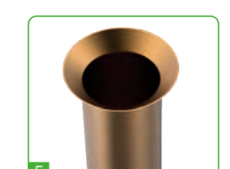
5 Finalize of expanding 45° copper pipe
