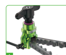
1 The expansion strip is inserted into the expansion body
