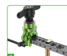
2 The copper pipe enters the hole, and the limit plate is on the copper pipe
