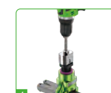
4 Or use cordless drill for fast flaring
