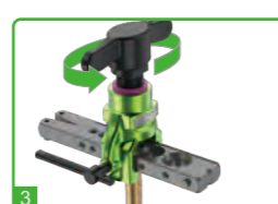
3 Slide the expanding body to the corresponding hole
