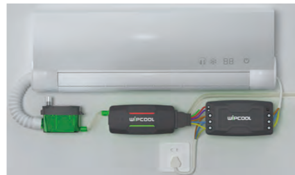
Failure drainage status Output was cut off when water reaches alarm level to trigger safety switch, To prevent refrigeration equipment continue to generating the condensate water
